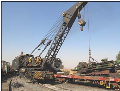
The only thing missing here is smoke issuing from the vertical boiler. Still, with nothing to be ashamed of, the compressed air powered crane makes short work of lifting this donated lathe from the flat car.
