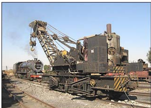
This old crane raises her boom in the sunlight after months of safe but shadowy under-cover storage on the end track in our depot. All the bearings, pivots and the slew rings have been kept lubricated and the old crane swung into position with ease.
