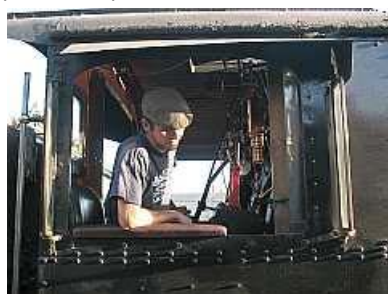
F08 - Are all the wheels still on? Loco-Minder Pat Ackerman was given the regulator for the afternoon shunt. Here, he confirms that the radius rod is lifting as he puts the locomotive in forward gear.
