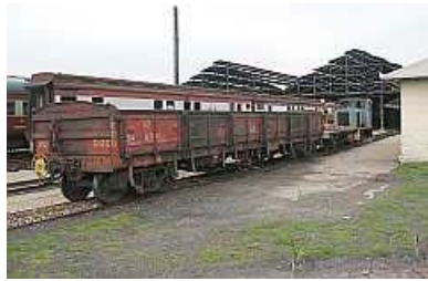
M02 🚛 An unusual visitor. A drop side gondola, colloquially known as a Dee Zed (DZ), even though this one is actually a WZ , waits in what has become our coach yard. This wagon was used to transport good quality coal from Friends of the Rail's Capital Park depot.
