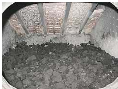
F02 - A fresh bed of fir starting coal in a Class 15CA firebox.
