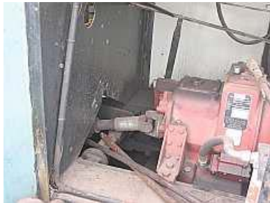
M07 🚛 Diesels never go wrong, right? Our old Hunslet Taylor switcher got stuck on the back tracks when the transmission drive coupling and pilot bearings disengaged.
