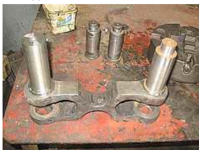
L01 – A pair of blank pins rest on a Class 12AR union Link. You can see the original pins in the background.
