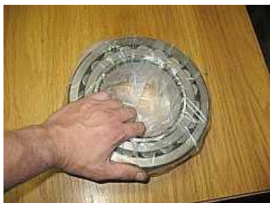
S01 – Zero miles on those rollers! A brand new double taper axle bearing, still in the original grease, for the Sandstone Estates GMAM Garratt No.4079 Lindie Lou. A bit too heavy to be used as a paper weight.
