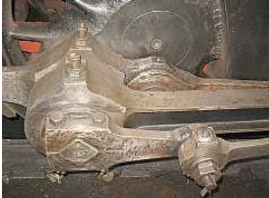
M05 🚛 Locomotive astrology 🚛 what happens when the planets, er, rods, all line up? The Class 15CA No.2056 🚛Corothy🚛 is resting with a coupling rod, a connecting rod and a return crank all neatly in line. (Note that this is not BDC.)
