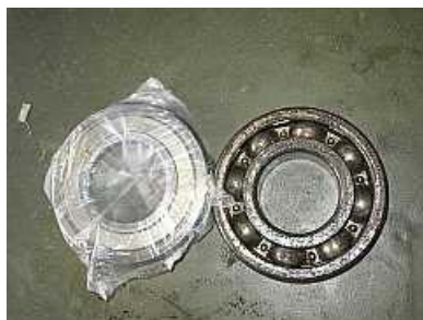
S02 – Something old, something new, something borrowed (the GMAM Locomotive!) and something that hopefully never turns blue. (From overheating.) This is a pair of Standard Stoker's Mechanical Stoker Crankshaft Bearings.
