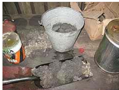
F03 - Fire starter kit. Soiled cotton waste is being soaked in paraffin in the shovel and being stored in the bucket. We just keep forgetting the matches as only a few Reefsteamers smoke.
