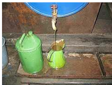
F05 - Now, the green oil goes into which jug? The decades old ritual of topping up the oil bottles for the road - the green cans being for the viscous green steam oil. We already had an oil can heating up on the flame plate - as this treacle-like stuff is otherwise too thick to flow into the lubricators.
