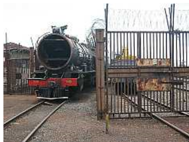
C02 A 12AR stripped for tube replacement is pulled out alongside the coal grab (visible through the gate) to transfer coal from the tender.
