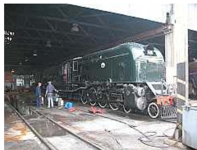
S03 – The rear unit of the Sandstone GMAM Garratt looks out over the Bissel Servicing area. We are working on the front engine unit of Bissel truck but the Bissel truck on this rear engine unit is to be overhauled as well.
