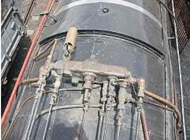
M04 🚛 Not a common sight a steam locomotive's turret manifold viewed from the cab roof in bright sunshine 🌞 and no electric wires in the way! This is the turret manifold, valve spindles and whistle assembly of our Class 12AR No.1535 🚛Susan🚛
