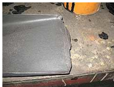
F06 - The bane of the fireman - the bent, worn shovel lip. This adds to thrust required to pick up scoops of coal, particularly when stirring the coal around the tender and one doesn't have a flat surface to scoop against. A few minutes in the vice straightened things up.
