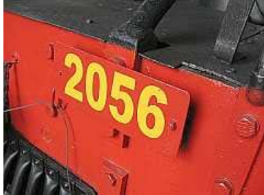
M06 🚛 This is one of the finished pair of off-set number boards fabricated by Fred Sewell for the Class 15CA. The handrails and braces on the locomotive prevent the fitting of a conventional number board directly onto the buffer beam.
