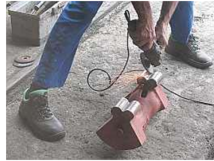
B09 The unusual geometry of the swing links (Upside down) ensures that the Bolster Plate is supported at the same height whether the locomotive is on a curve or a straight track. They are ingeniously designed so that when they are tilted at an angle, the circular lobes on the underside engage and jack up the quadrant to make up the height that would be lost in the diagonal movement.
