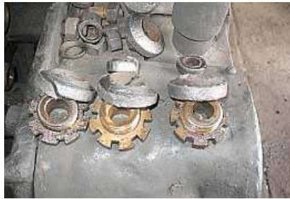
S08 An array of piston rod glands and the castellated gland nuts lay spread out on the cylinder cladding. Notice the correct helical gap in the gland seal on the left.
