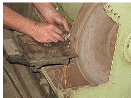
B06 ☞ The Countersinking Keys are being ground off the bearing bolts on the large grinder. You get an idea of the size of this machine by looking at the scale of the hands and the grinding wheel.
