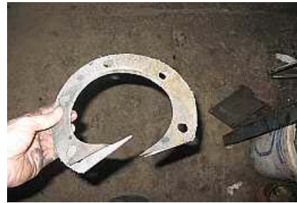
S09 A newly fabricated gasket for one of the two crankcase end covers.
