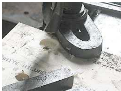
B05 ☞ A close up of a newly drilled countersunk hole next to a standard bore. This is actually much cleaner than it should be, as the characteristic very long curly Vesconite shavings have been removed.
