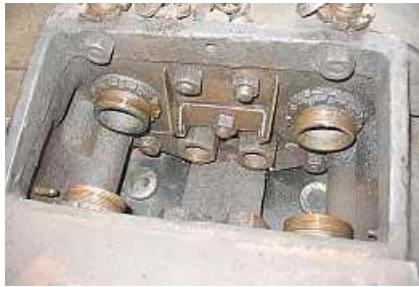
S07 View of the empty rod chamber after the pistons and valve spindles have been removed. The valve rod apertures are the two smaller ones in the center.
