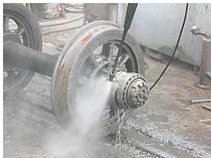
A02 A high pressure water wash in action. Care was taken not to over spin the bearings although the drag of the displaced outer races acted as a brake anyway. The bearings would later be washed with a mixture of degreaser and diesel fuel.
