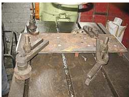
B04 ☞ The two new blank Vesconite plates clamped with one of the original slide plates as a template for drilling.
