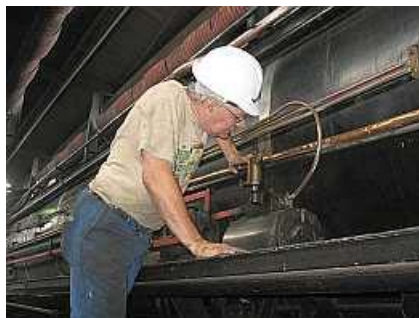
G02 Johann Breydenbach visually checks the glands for the Power Reverser's Actuator Cylinder's Valve Chamber. He's resting his left hand on the Displacement Lubricator and is actually looking at the gland for the 1/4 inch steam supply line for the cylinder.
