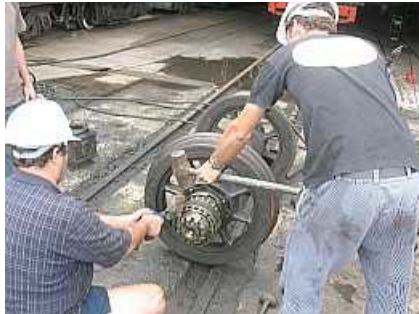
A07 ☞ The first attempt to get the castellated retainer ring off. We were very wary of the possibility of hurting someone in this operation.
