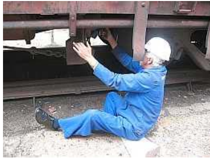
W02 ☹️ Safety Officer Cliffie Mathee spent the day inspecting handbrakes on the rolling stock. Here, he is lubricating the very stiff handbrake gearing and chain pulleys on the Friends of the Rail NZ Gondola. His left hand is on the quadrant block and you can see the actuating chain angling up to the left.
