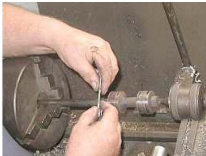
S10 James measures the thicknesses of Valve Ring grooves while spinning the spindle on the lathe for cleaning.
