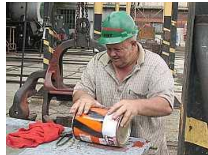
B12 The Bissel Frame is painted. Piet Buffels Steenkamp stirs up the primer by rocking the tin on the Komati box.
