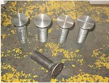
B07 A row of newly fabricated countersunk slide bearing bolts stand to attention behind the fallen original bolt used as a sample.
