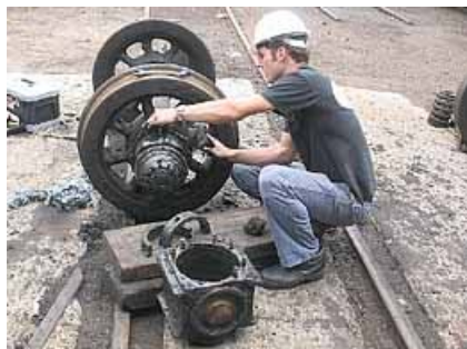
A01 Patrick Ackerman is scraping off an axle box back end. The axle box lays seal end upwards in front. Notice that two of the studs got left behind in the back plate. The blocks of wood were used to stop the box from turning. On top of the wood are the semi-circular intercostal spacers for the two outer bearing races.
