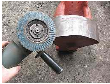
B08 The useful emery flap grinding wheel used to polish up the working faces of the swing links, the radius ramps and bearing surfaces of the sliding Bolster Plate.
