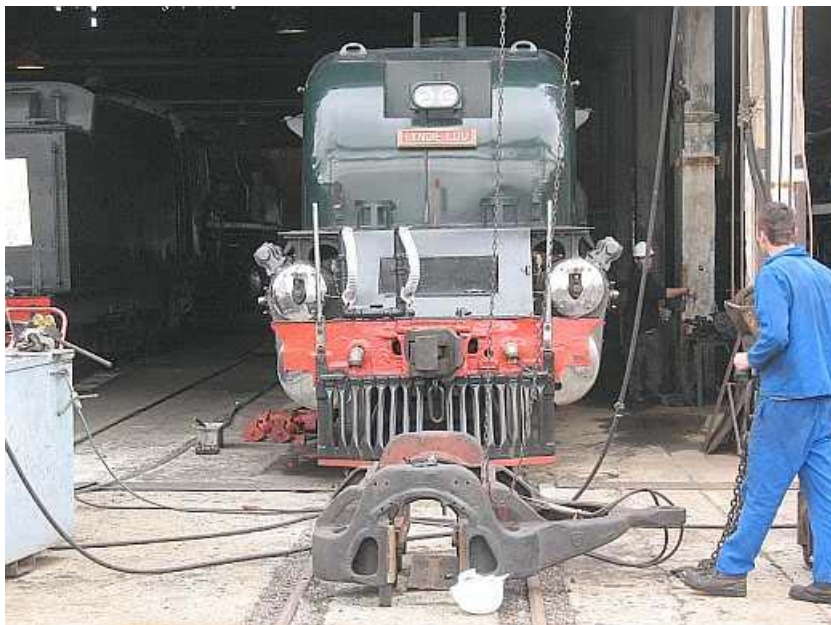
FP01 Fixing the parts to enjoy the whole. (A very big whole ) The leading engine unit of the Sandstone Heritage Trust 's GMAM Garratt No.4079 Lyndie Lou oversees and approves of the Saturday Bissel Truck assembly project.
