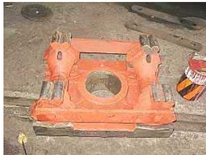
B11 The Bissel works. (Albeit upside down) Here you see the swing links, connecting bars and the Bolster plate assembled as they would have been within the Bissel Frame.
