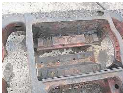
B02 ☞ The rather crusty interior of the Bissel Frame with one slide plate (top) removed and the lower slide plate still in place. Notice all that corrosion evident where the top plate was. You can see how the lower plate is distorted and pushed inwards at the top edge.
