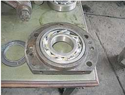
S01 New Crankshaft Main Bearing installed into one of the crankcase end housings. It's merely an interference fit no press was required to insert the bearing.
