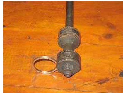
S12 A newly machined valve ring blank engaged in a groove on the valve spool. The ring's slot hasn't been cut yet.
