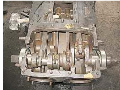
S03 Top view of the open Crankcase with all internal components installed (except the left hand big end bearing cap)
