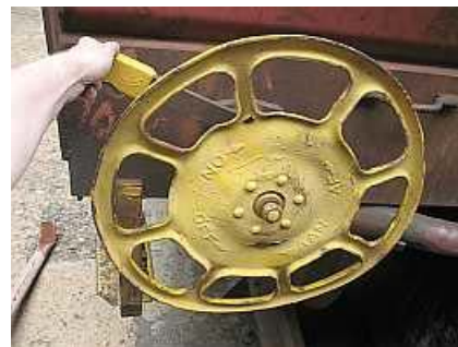
W06 ☹️ Lee and Cliffie test a handbrake quick release lever. This one was totally disengaged and the one on the other end won't move ☹️ this beat old wagon needs some serious maintenance!
