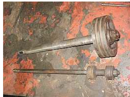
S06 A removed piston and valve spindle. The piston has been roughly cleaned but the valve spindle is as-removed. Notice that the valve ring slots, of which seven had NO rings, have filled in with corrosion.
