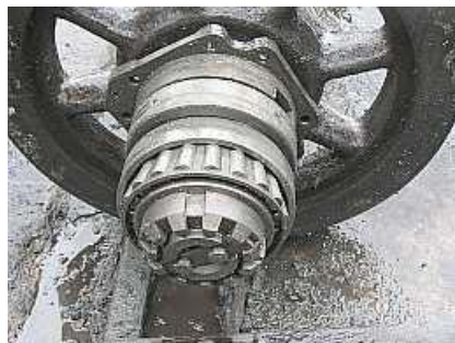
A03 A freshly water-cleaned bearing glistens under the oily droplets. Notice the almost horizontal split pin holding the castellated retaining ring in place.
