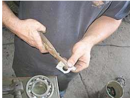
S02 Cutting out new shims, using an original brass shim as a template.
