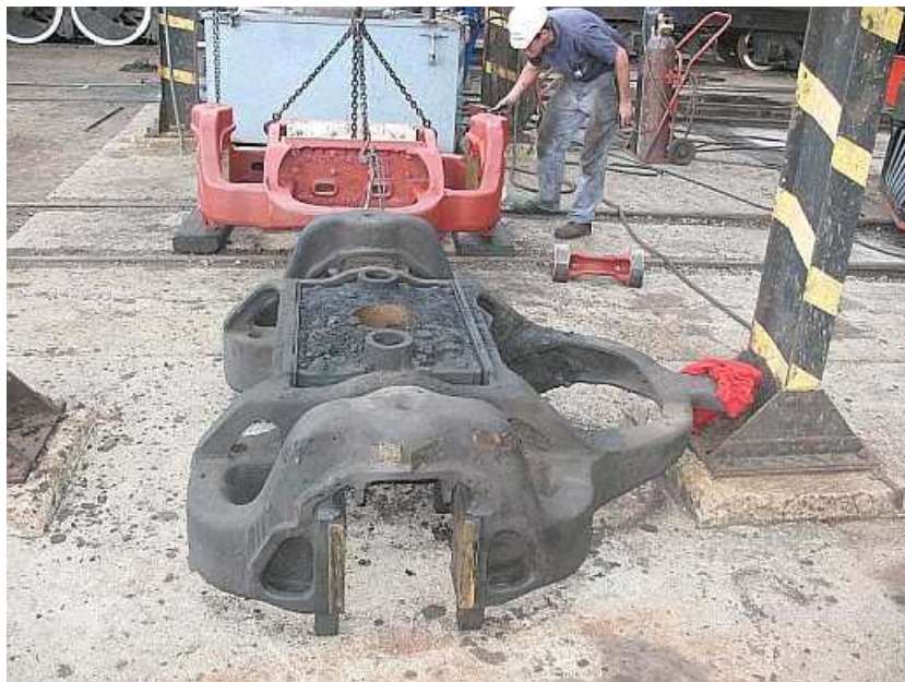
FP02 Comparison. The original rear engine unit's Bissel frame in front of the original front Bissel's frame undergoing assembly. Once the GMAM Garratt is running again, we'll clean this frame and free up the seized Bolster Plate before putting it into storage.
