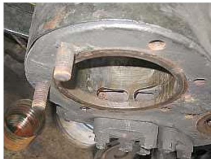
S05 A view of the steam ports in the cylinders. The valve chamber covers still need to be removed. Notice the two cylinder head studs still seized in place. Michael cleaned and serviced each one of the studs.
