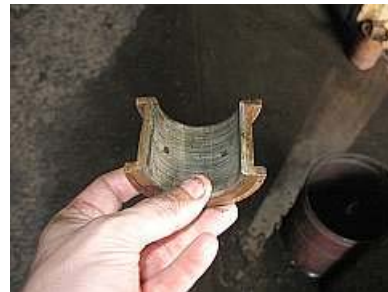
S03 A worn and scored Big End Bearing.
