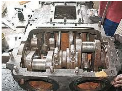
S01 The Stoker Motor Crankcase being stripped. It's a two cylinder engine. The two con rods remaining in the center are for the valve gear eccentrics. You can just see the big end of the left hand rod lying prior to removal.
