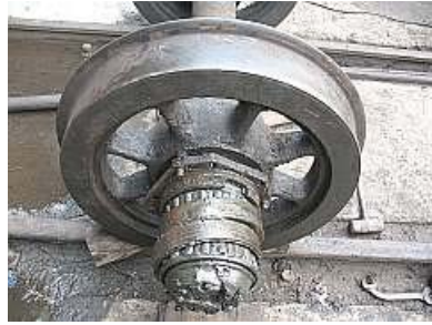
P11 An axle box surprise. An older self adjusting bearing is revealed as Kerry and Jaun removed the axle box on the original axle.
