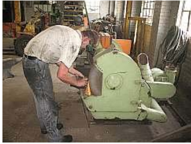
P10 One of many trips to the grinder to put a new cutting edge on the chisel used to split those very hard bearing races.
