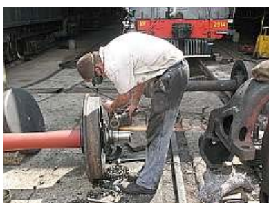
P07 A goggle eyed alien, who bares more than a passing resemblance to Shaun Ackerman, tackles the splitting of hardened steel bearing races with an angle grinder.
