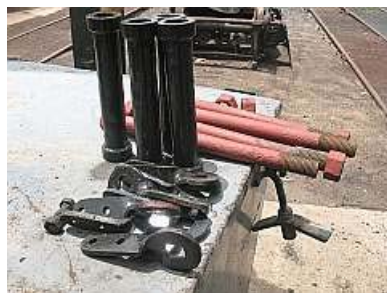
P05 A spread of cleaned and primered removable Bissel Truck parts.
