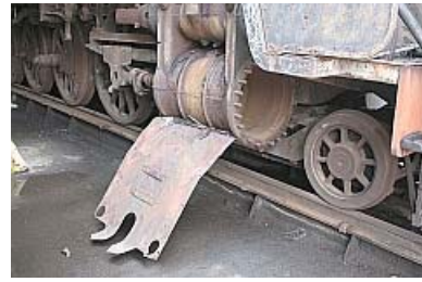
M03 A Class 15F Locomotive in the dead-line shows a clean set of cylinder castings behind a sprung and fallen cylinder cover plate. The total lack of the usually messy looking insulative lagging shows the complexity of the cylinder and valve chamber castings works of art.
