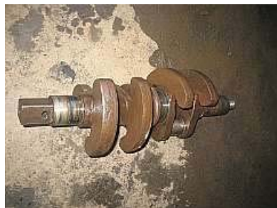
S05 The two-throw Journal Crankshaft with one of the valve eccentrics visible. Notice that the cranks are 90 degrees apart to avoid the situation of having both pistons at dead center and thus a motor that won't start. (A steam locomotive's crank pins are set up the same way.)
