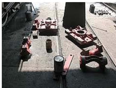
P02 Some cleaned and painted Garratt Bissel hardware from last week with rusty threads from being left in the rain. Those strange looking twisted brackets in front are for the Bissel oil cups.
