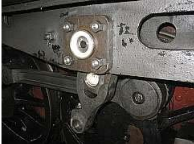
M04 Class 12AR No.1535 Susan now sports expansion links and die blocks with eerie looking shining white custom-made Vesconite bearings.
