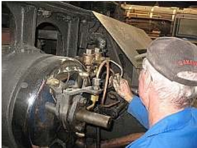
M07 Tony King gets to grip with the myriad pipes and fittings of the Garrett's pressurized lubrication system. He's remarkably patient with Brasso and a rag.
