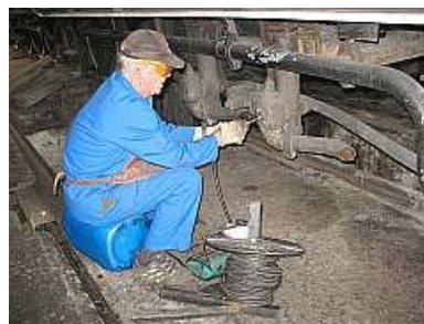
P03 Tony King gets to play with some flexible shafted power-toys. He's busy cleaning the dirt from the GMAM Garratt's injectors.
