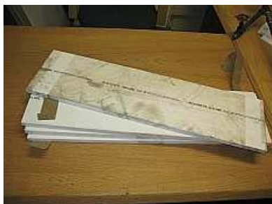
P04 Hi-Tech breadboards. Four sheets of HiLube Vesconite as obtained by Shaun during the week. These are to be used for the sliding surfaces on either sides of the bolster plates.
