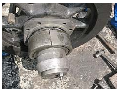
P08 An inboard outer bearing race that has been grooved just prior to some delicate hammer and chisel work to split it.
