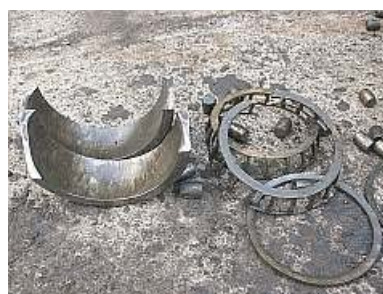
P09 Rest in pieces. A scatter of dead bearing parts. a split race, two bearing cages, a spacer ring and a generous sprinkling of bearing rollers.
