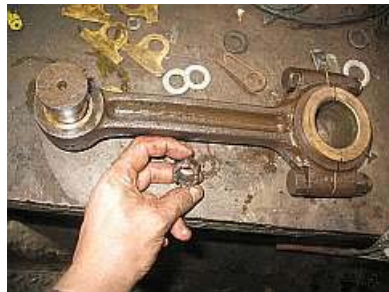
S02 Stoker Connecting rod being dismantled on the work bench. Here a badly worn big end cap nut is being examined. Those brass shims at the top left fit between the big end cap and the connecting rod.
