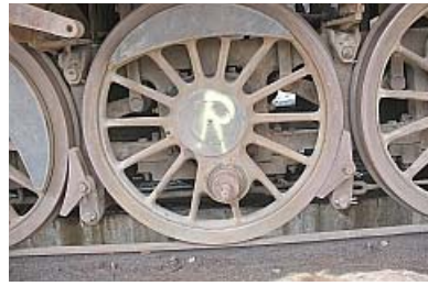
M02 The dreaded capital 'S' spells an engine's end as condemned for Scrapping. Here is an 'R' for 'Retain' or 'Reserve' on the wheels of a Class 15F loco otherwise marked up for cutting.
