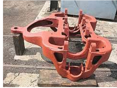
P12 The stripped and primed donor Bissel's frame waits patiently while it's components are stripped and overhauled.
