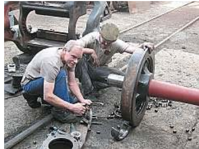
M08 Andrew King (front) got a bit teed off towards the end of the day. It was one of those days where he is constantly getting interrupted and asked for advice and he got none of his own work done. Here, he feels better getting a puller ready to pull a bearing back plate off an axle.
