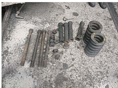
P01 A choice assortment of dirty axle bolts, sleeves, springs and nuts wait to be cleaned, lubricated, primered and then painted..
