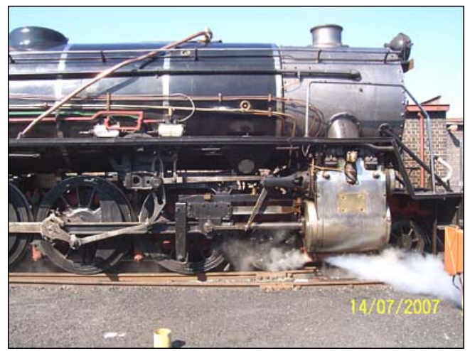
Rear top-dead-center - RHS piston . The radius rod sits in the center of the expansion link while the cylinders blow steam through the cylinder cocks. Those running boards are head-high to a 6ft man - impressive for a "Cape Gauge" Locomotive!
