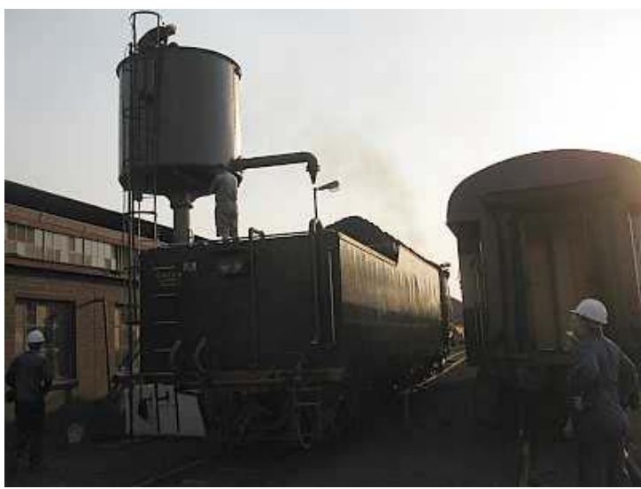
FP07 - The first attempt at using the water tower is interrupted when the tank's water supply is switched off and the ball cock is removed to bend the float arm downwards. Consuming 18 000 to 33 000 liters of water at a go in a tender or a water tank car is costly enough without water running to waste all day. The water level was slightly too high and the tank was set to overflowing when the float started bouncing.
