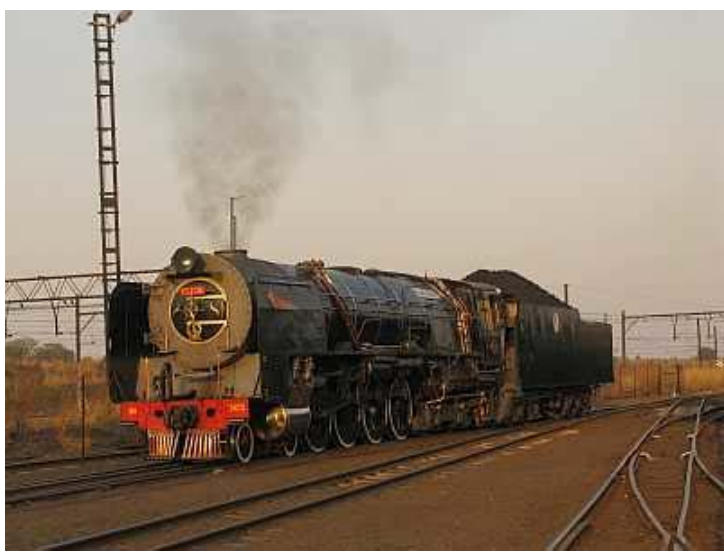
FP15 - As she rolls back after putting the coach properly away under the cover of the old running shed, a loafing "Elize" shows the V-shaped exhaust that is characteristic of the Class 25NC. (LG)
