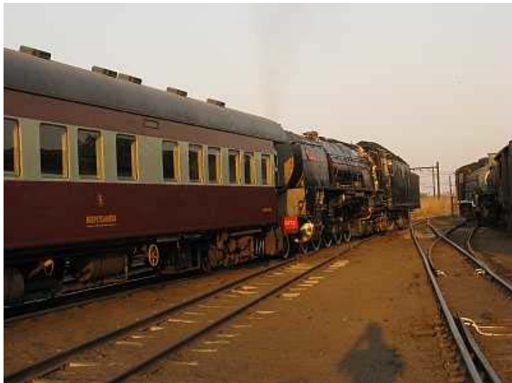
FP13 - The mighty locomotive hardly feels the weight of the single 40 ton coach as the shunt move pushes over the newly concrete sleepered track. The fireman is nervously running the injector for the first time of this shunt and after a blown gasket was replaced in the outer delivery pipe flange. He'd also fitted a proper square shank to the water valve and extended an old injector water valve handle and shaft to suit - so now the originally loose fitting valve truly does open and close fully through the 90 degree operating arc of the valve handle. (LG).
