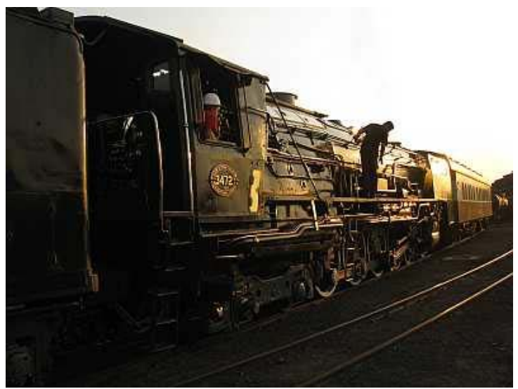
FP12 - Having just coupled to the coach, the Class 25NC No.3472 "Elize"; pauses with her rods down while the fireman checks the blowing gland on the rear of the power-reverser's actuator cylinder.
