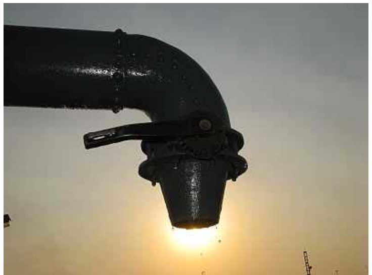
FP10 - Feel the pain! The truncated pipe came out fairly neatly and there is still enough of the cone left for us to put a drop bag on in the future. Excepting the plinthed A-Class, all of our tenders have centralized water hatches, so it isn't really necessary.
