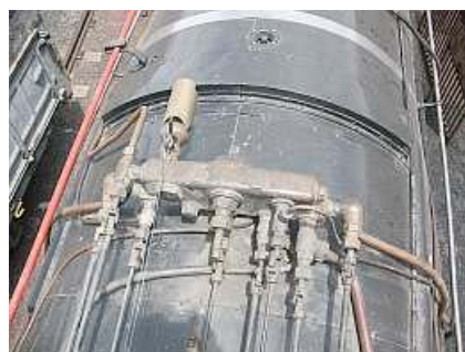
B15 The turret manifold, valve spindles and universal joints of the Class 12AR. The 15F's have a two piece manifold which is closer to the cab but the principle is exactly the same.
