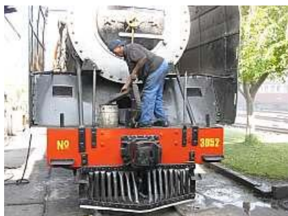
F01 Sakkie wields the short-shovel to clean up the leftover smokebox char from the front deck. This turned out to be well timed as this was the area upon where the brake vacuum pipes would be removed later on that day.
