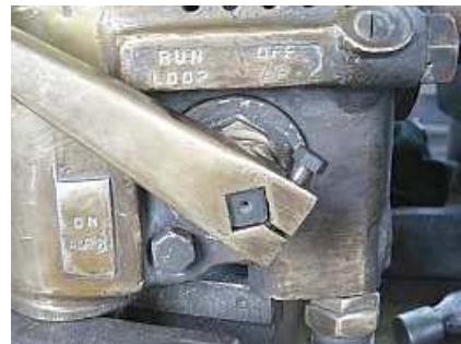
E15 Detail of the end of the brake lever. Notice the annotated three positions of the lever. (Off \ Aff) (Run \ Loop) (On \ Aan)
