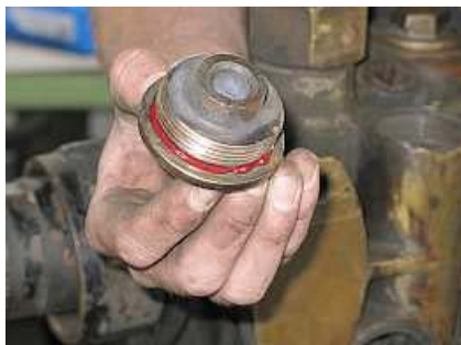
E05 Installing a valve cover. Notice the fresh red bead of LockTite thread locker fluid being used as a high temperature cap sealer.
