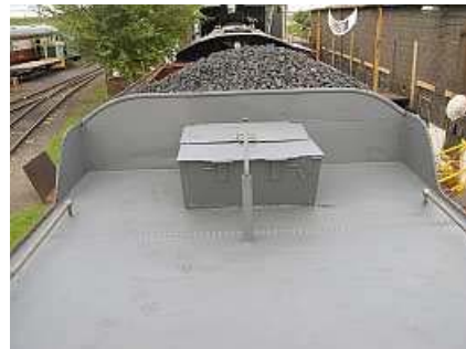
L12 ☞ Freshly painted tender deck doesn't actually gleam in the sun, but looks a lot neater and should help prevent future corrosion.
