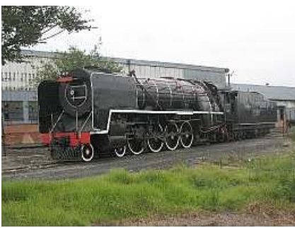
L01 ☞ Avril in her as-delivered paint scheme. Note the plain black un-badged SAR style smoke deflectors and the custom bulls-eye driver wheels. Also notice the lack of a cab number plate and wing heralds.
