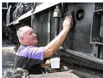
F06 (Prev week) Oom Attie cleans the left side of the fire box with his secret blend of oils, wax and paraffin. This is a tricky area to clean on a live locomotive because of the heat, and that very hot injector steam line.
