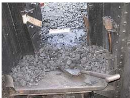
F02 The shovel plate after the first helping of coal. Looking through the coal doors behind the front heap, you can see that the stoker slides are all closed. The gobble-hole is buried two slides in the heap at the rear.
