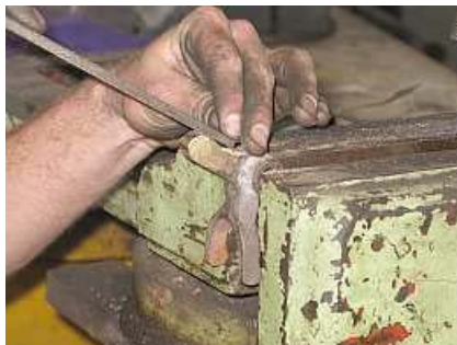
E14 The cam follower is being carefully re-profiled to bring the valve lift back into spec.
