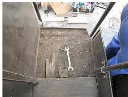
F09 Two planks came up on the driver's side, revealing rotten cross braces, termite dust, splinters, coal dust and fluff. You're looking down at the steel under tray after cleaning, but before the angled step cap was removed.
