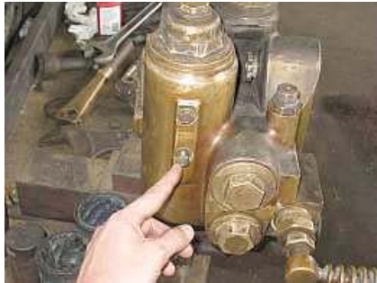
E10 One of two valve seats retainer bolts that have to be carefully cut and machined to fit against each valve seat exactly. (The ejector is upside down in this picture.)
