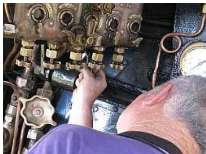
F07 "Picasso de Necker" paints behind the lubricator. Notice the five sight glasses a characteristic of a mechanically stoked locomotive oil being fed to the two valve chests, the two cylinders and the stoker steam intake. (A hand bomber's lubricator only has four sight glasses.)
