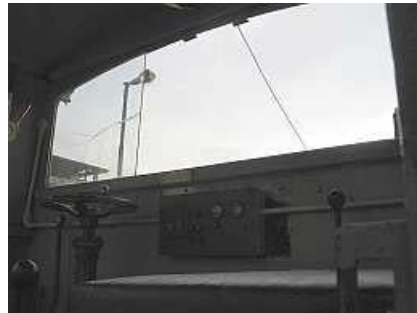
G02 📷 Interior view of the windscreen area. Only the (cracked) left hand pane still remains. The lower slide arm can be clearly seen above the instrument panel. The square glass pane actually extends beyond the curved aperture as visible at the top left.
