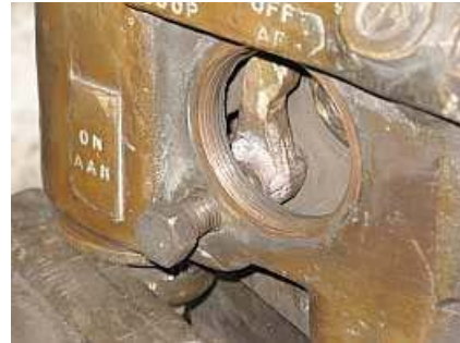
E12 The valve lifter after being wrangled home and the pivot pin has been half installed. The valve is heavily spring loaded, which added to the fun.
