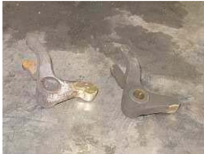
E11 A rebuilt valve lifter \ cam follower is shown to the left while the worn unit from Avri's ejector is shown to the right. No wonder the air valves weren't opening.
