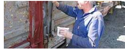
C03 📷 The master starts with the convoluted sections first. Notice he has his tongue out in concentration as he fills up all the nooks and crannies with the oxide red paint.
