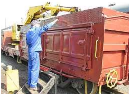
C04 📷 The roller finally comes out for the flat panels and the plate work. The size of the photos doesn't really show how smooth the paint job is.
