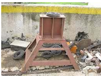
M07 One of the carriage jacks (With a padding disk) in storage at the Shongololo Express Tracks. These jacks are used to drop the bogies from under the coaches.
