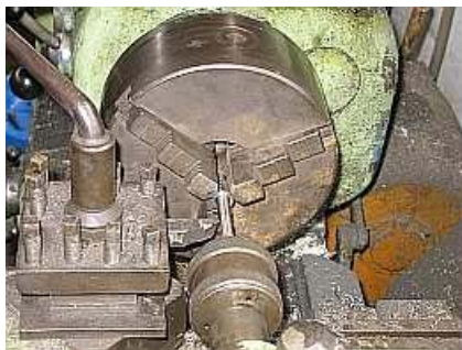
E02 The new lifting pin is being turned down from 15mm stainless steel stock on the lathe. That small hex-head took some centering before the bolt would spin straight in the lathe's chuck.
