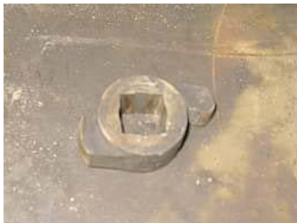
E13 The removable cam. You can just see one of the re-dressed cam profiles at the lower left.
