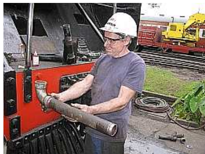
B08 The troublesome buggler and I don't mean the Chief Engineer. Andrew King sarcastically holds out the newly cut and threaded dropper pipe.
