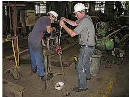
B06 Andrew acts as a skilled self-adjusting counterweight while Lee takes a turn at the thread cutting. Note the tub of lubricating oil on the floor.
