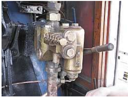
E19 Newly installed brake ejector. The top pipe is the steam inlet and the bottom pipe is the vacuum line for the train's brakes. You can see the T-junction tap off for the duplex brake vacuum gauge. The small pipe at the lower back leads to the locomotive's vacuum cylinder. Not visible, coming in horizontally through the back, is the steam, entrained air and vacuum discharge lines which blows to waste inside the smokebox.
