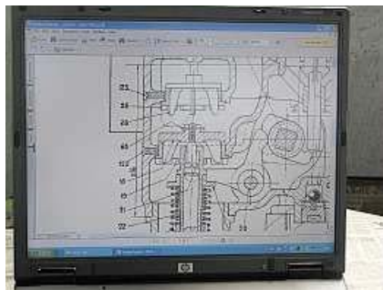
E01 A blend of modern technology and vintage machinery. Here's a CAD drawing on an ejector vacuum valve. The L-shaped object in the center is the valve lifter and the cam is clearly visible middle-right.
