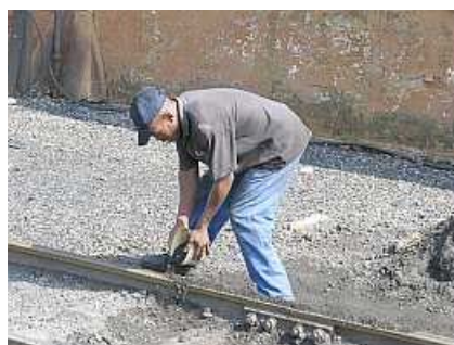
M08 Sanding rails the old fashioned way. Attie and Sakkie battled to get the Class 25NC 3472 Elize and the Class 15F No.3052 Avril swapped over on the wet, uphill yard lead. The Hunslet Shunter has no sanding gear/.
