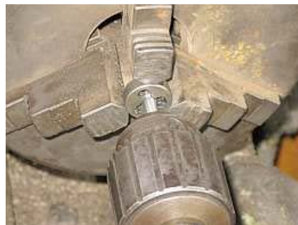
E03 Cutting the threads by hand, using the lathe chuck as a hand-powered die-nut spinner.
