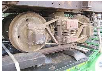
S02 (Prev. week) A classic arch-bar truck complete with quad coil springs. Note the wooden bolster beam and the unusual plain-bearing boxes.
