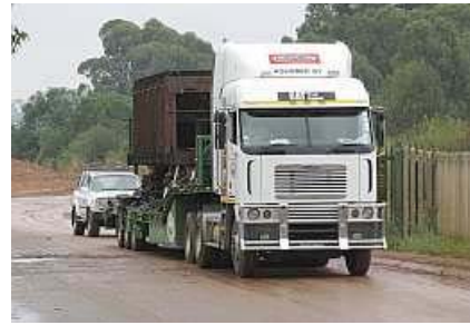
S03 (Prev. week) On the move at last. The Sandstone Estates Freight Liner low-bed crawls cautiously out at about 20kph not because the load was too heavy, but because it was potentially top heavy even with chains.
