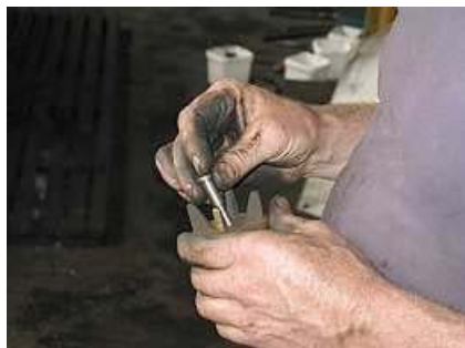
E04 Test fitting a new valve limiting pin. The wider head prevents the valve from lifting so far as to disengaged the guides from the seat when operating.
