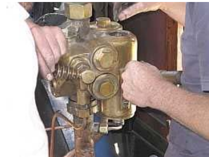
E23 Hunt the Hitch. A hopeful search for a classic dumb mistake or perhaps some dirt that got into the injector.
