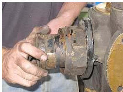
E07 The new vacuum union is being screwed in by hand - testimony to the cleaned reconditioned threads. Note the retracted union nut which is
