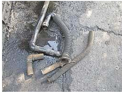
B02 A collection of cut up and dismantled brake lines. The black painted pipes are the exposed pipes for the brake stand. The angled pipe at the bottom right is the cross pipe between the running board and the center line. The rusty pipes are the dropper from the running board height to that of the front buffer.
