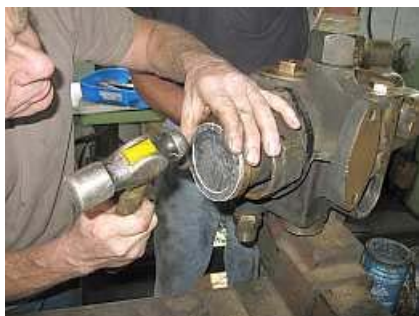
E08 In one of the many positional adjustments of the ejector in the vice, Andrew finds a convenient angle to opportunistically tap out a new gasket
