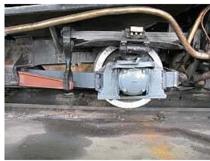
L03 ☞ Grey painted Bissel truck. Notice that this engine uses roller bearings on the trailing axle. The red painted beam to the left is the compensating beam.
