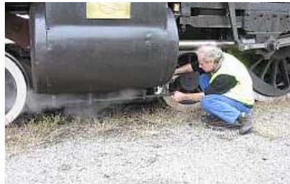
F21 ☞ Andrew King is trying to spread and straighten the U-shaped coupling at the end of the rod in situ. The rod had to be removed to finish the job.
