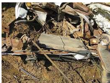
S10 The tank crew did a sloppy job. The steering box, headlamp cup, steering column, cooling ducts and hoses, and amazingly, the radiator, had survived two tank passes.
