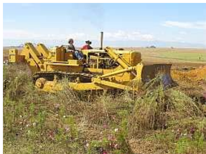
S07 Sandstone Zamboni. Instead of scraping ice from an ice rink, the Sherman Tank's playground was straightened after every two or three runs by this vintage caterpillar Bulldozer. Those poor cosmos flowers looked rather battered by the end of the day.
