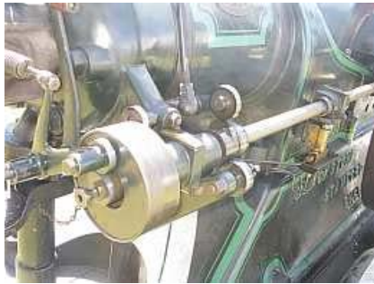
S20 ☞ The fascination of an ☞open☞ engine. How many cams do you see in this picture? Including the lubricator at the right center ☞ there were four cams steadily clacking away.
