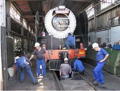
W01 A very busy Top Shed. There are three teams represented here. The cleaning \ painting crew the locomotive roadworthy inspection (standing in pit) and the helmeted firefighter high-stepping in from the right.
