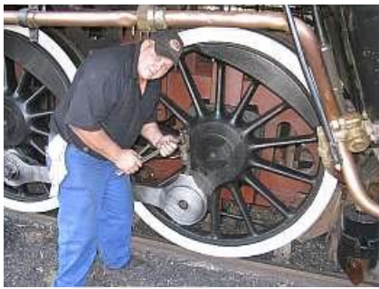
W16 📷 Piet 📷Euffels 📷 Steenkamp greases the left rear driver wheel while the bearings are still warm even after a short run. Note the beautifully shiny coupling rods.
