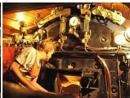
W23 📷 Lee Gates adds a few more bites of coal to the leading edge of the coal bank 📷 a panoramic self portrait from the top of the locomotive's tool box.
