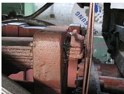
W04 A freshly oiled spring hanger bears testimony to the thoroughness of the roadworthy and preparatory lube work.
