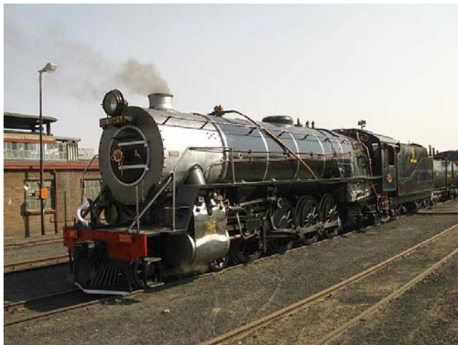
FP01 - Connected to three coaches and drawing off the air in the train vacuum brake lines, a clean Class 15CA No.2056 "Dorothy" looks good as she sizzles gently to herself in a rare calm moment on this blustery dusty highveld day!
