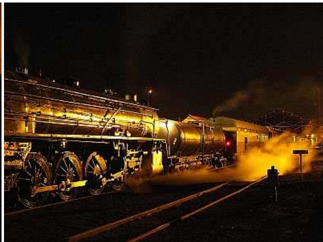
FP16 - Less than 2 minutes to departure. Pushing the train out the yard and backwards along the main line is characteristic of a Boksburg East start as there are no turning facilities there. After a short haul to Boksburg, running tender first, the loco will run around to the front of the train, and will be facing the right way for the westbound run to Magaliesburg.
