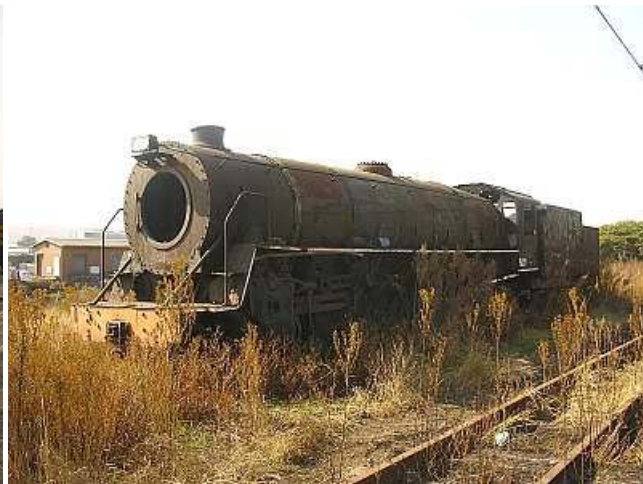
FP02 - Hard to believe this rusty wreck is of the same series and class as our well loved "Dorothy". This locomotive was officially set aside for preservation but was never taken into a place of safety. Some scrap metal bandits sealed its fate but cutting the frames away (with a hacksaw!) and extracting the valuable axle bearings for sale as scrap.
