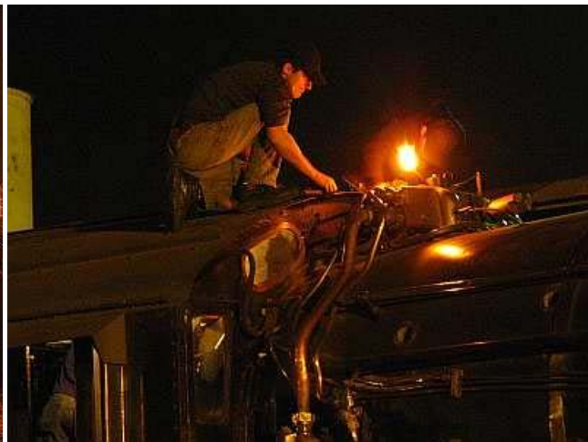
FP14 - A turret valve's universal jointed shaft has jammed up. Dawie (Trainee - left) and Andre (Fireman) free up the shaft and adjust it to make sure that it won't jam on the trip. (You can't mount the cab roof under electric wires!)
