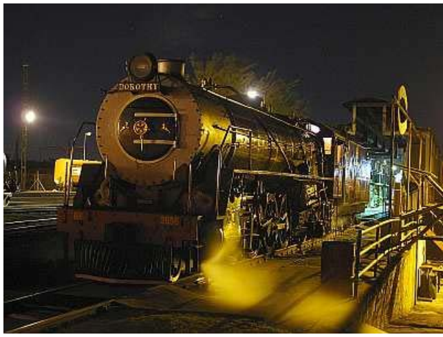
FP11 - Sizzling on through the night. It's 1am on Sunday morning and boiler pressure is stable at 950kPA with a drowsing, banked fire. An issue with this locomotive is the slightly leaky regulator which means that you can't really "button up" the boiler for the night. A refreshing cold front has just passed, with an excitingly blustery wind and I've just had a representative of the overnight caboose gang shamelessly begging for my chocolate.
