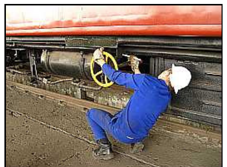
C03 – Coenie catches the end past the vacuum tank and threads it over the handbrake wheel shaft.
