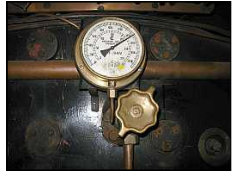
T06 – A strange sight. The back head pressure gauge is mounting up even though the water glasses have been removed and blanked off.
