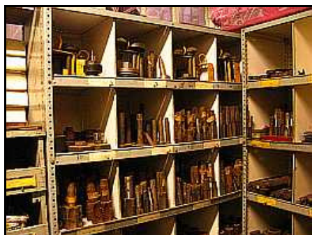
D04 – Just a small selection of the antique steam locomotive tools recovered from the Millsite Workshops. The top shelves have valve seat grinders – in their original stands. The lower two shelves are host to a selection of locomotive sized thread taps, reamers and thread chasers.
