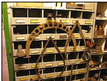
D05 – Check out these callipers and that locomotive-sized outside micrometer.
