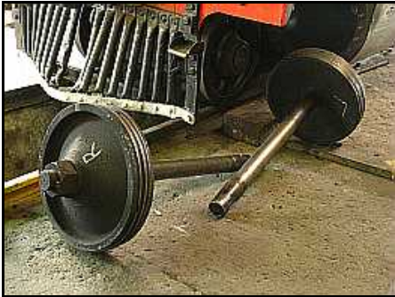
P01 – A pair of withdrawn pistons wait for stripping, cleaning and groove machining. They are attached to the crosshead by wedges passed through slots, hence the lack of readily visible fastener hardware at the end of the piston rods in this photo.
