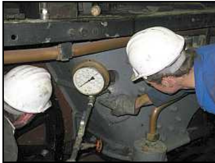
T05 – Patrick and Shaun discuss the regulation of the test pressure. Patrick has just, inevitably, succumbed to the temptation to tap the test pressure gauge.
