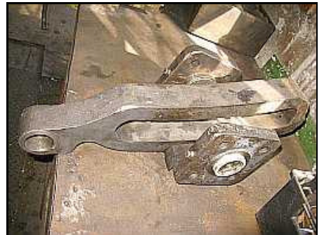
P06 – A removed expansion link waits to have the bearings modified. The valve gear of this locomotive is to be completely refitted with Vesconite, just like our successful Vesconite conversion of the Class 15F No.3016 'Gerda'
