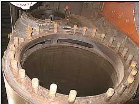
P04 – A worm's eye view of the front steam ports at the front of the double acting steam cylinders of this 12AR locomotive. There is an identical set at the rear. These act as both intake and exhaust ports, the function being switched by the piston valves.
