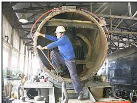
E05 – The extension bar is just long enough to clear the smoke box and Dawie has free room to swing the tommy bar to rotate the extension. He caught his knuckles a few times on the protruding studs. In this pic, he is just about to turn the tommy anti-clockwise.
