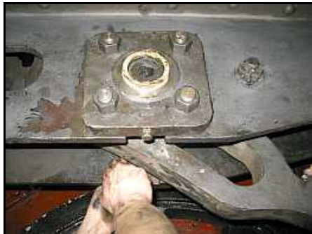
P05 – James Thomson and Juan 'Nippies' Buys installed the expansion links three weeks ago, with new white vesconite bearings in the trunnion bearings.
