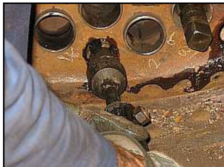
E04 – The tap in action with Patrick using both hands to keep the shaft aligned. The streaky black marks are oil drips and the square shank at the top right is a spare tapered tap lying loosely in a tube.
