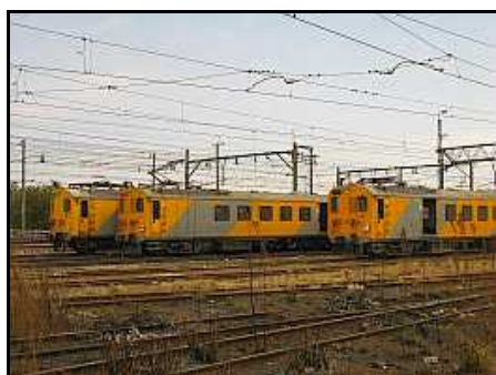
M04 – A brace of 5M2's snooze the Saturday afternoon away. Note that the center unit still has the pantographs up and is still energized. The still-electrified but weed grown tracks in the foreground lead to a three stub-storage tracks that buffer up against a hardly used access road.
