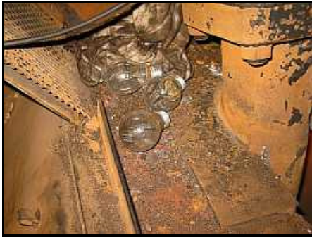
M07 – Patrick Ackerman's dead light bulb collection. These are 32V locomotive-standard globes and are the casualties of two Saturday's worth of smokebox work in the isolated-secondary 32V inspection lamp.
