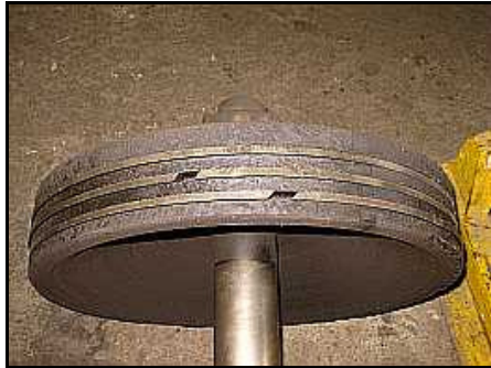
P02 – A close up of the three piston rings as removed. The rings are a little slack but not in too bad a condition. But they are going to be replaced anyway.
