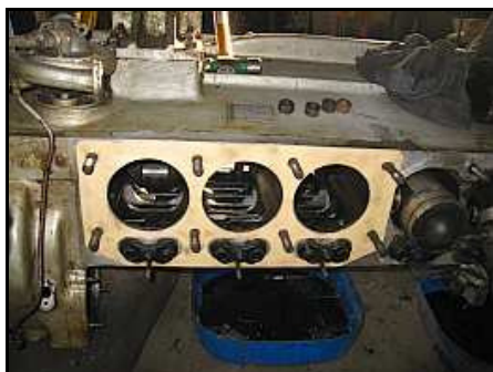
E08 – Freshly inserted crank case gasket. The pushrod guides have already been re-inserted. The object protruding into the left most cylinder is the exposed crank throw
