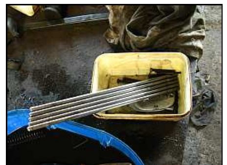
E21 – The newly cleaned and rather strange looking and feeling lightweight push rods. The missing rod number 6 is the faulty rod.
