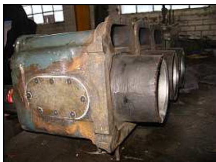
E02 – The oval end plate where the original coolant leak was, has been resealed with a gasket and with sealant. Notice that the eight bolts are actually allen heads – totally impossible to undo with the two engine blocks standing end-to-end on the crank case with about a 4mm gap..
