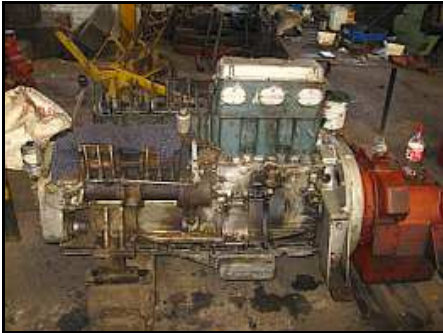
E16 – The engine is coming back together. One cylinder head has been installed with all valves, rockers and the decompression shaft. The sump has also been re-installed.
