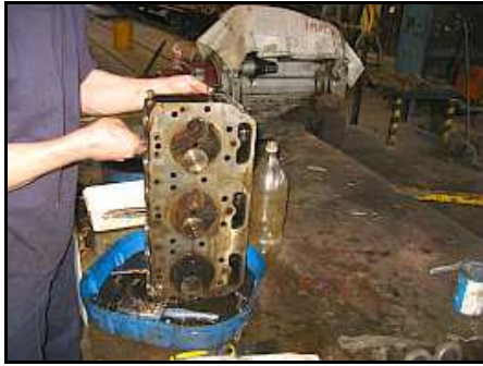
E21 – The cylinder head gets an afternoon bath. Notice how the larger inlet valves, naturally cooled by the induction mixture, came up shiny without brushing. You can see the fuel injector holes right between each set of valves.
