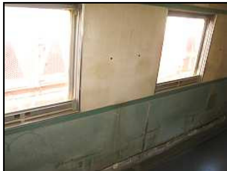
C13 – Courtesy of high-mileage Sandstone Coach No.25206, the tired original Union Carriage and Wagon SAR laminates after 30 years plus of service. The rough looking 'skirting' is actually the under plating of the original steam heating pipes, which have been removed.
