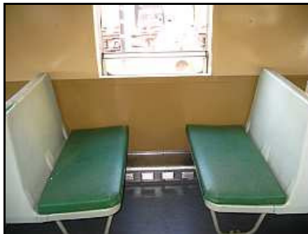
C14 – The new two tone paint scheme and the polished heater covers show to advantage here. The seats were fitted over the new flooring the previous day. Plans are underway to make Velcro-fastened slip-on padded covers for those hard-back seat shells.
