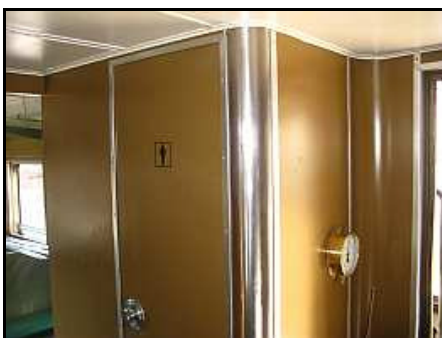
C10 – A freshly painted coach vestibule. Note a typical Dr. 'Smudge' Ackerman touch... the brass brake vacuum gauge had been polished before refitting. The 2-leaf gangway doors are still missing in this picture.
