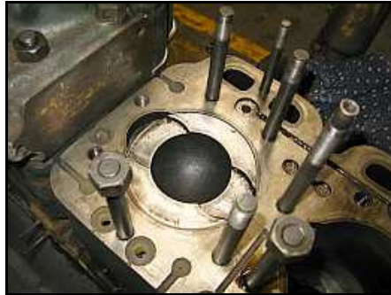
E17 – Top dead center. In practise, the induction air would swirl inwards in a toroidal pattern. (it is, colourfully, 'called 'squish') When the injector fires, right into the center of the cupped piston crown, the atomized fuel is well mixed into the rapidly heating and very turbulent air.
