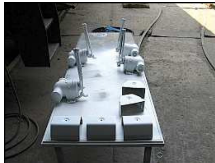
C15 – Painted coach parts after primer coat application. In the foreground are supports for the central lighting strips and the background are the four (non original) coach door closers.
