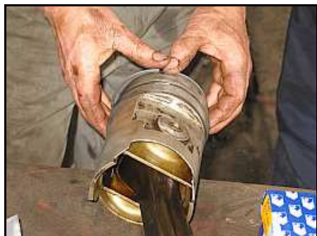
E13 – Inserting the new piston rings. The very wide top land meant extra care had to be taken in walking each ring down to their slot without snapping them. This is the top-most (easiest) compression ring going on. Note the massive fully braced construction of the piston skirt – typical of a diesel engine.
