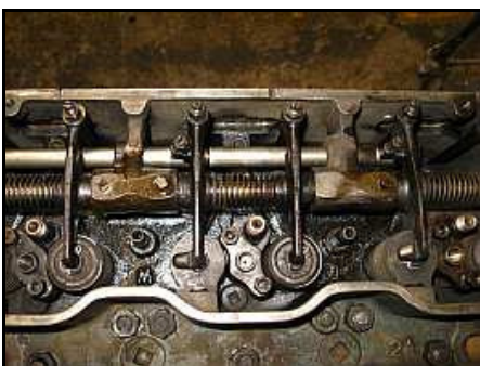
E19 – The diesel injectors have been installed and clamped down. The diesel fuel piping actually couples to the threaded clamp and not to the injector itself.
