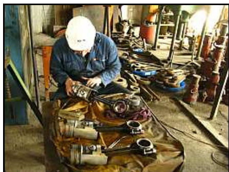
E07 – Aiden settles down scraping the carbon deposits off the pistons while avoiding longitudinal grooving and scratching of the alloy material.
