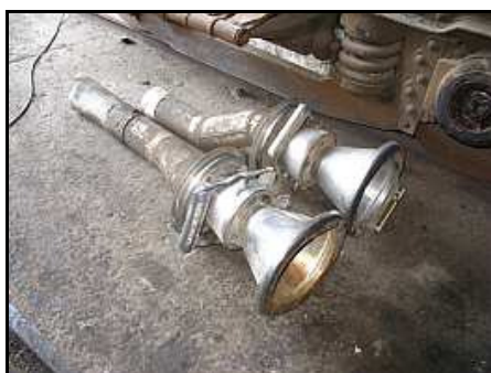
C04 – Two spare toilets with working flap valves and intact drop pipes wait for test installation to check the fit. Note the angled discharge pipes. The originals go into the spares stock.
