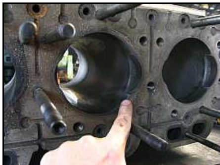
E05 – Here's a rather unusual valve pocket. You can see the carbon ring in the right most cylinder, which shows the position of the upper compression ring at Top Dead Center. The piston land actually 'covers' the valve pocket.
