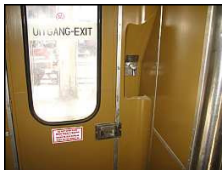
C11 – Details. The aluminium needs to be polished and the window needs a good clean. But notice that original style bilingual 'door leaning' decals have been re-applied, the latch is perfectly straight and all the aluminium is present.
