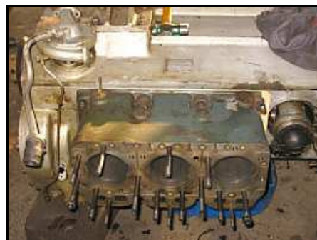
E09 – The block's revenge. Those deeply insert mounting bolts don't allow sockets – open ended spanners had to be used, 16 th of a turn at a time. This is when I chose to 'disappear.'
