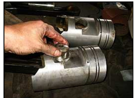
E12 – Installing the fully floating gudgeon pins.
