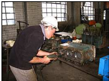
E04 – The carbon smeared unswept area of upper bores receive a good but gentle polishing with a home made flapper. This is the first cycle and you can already see the shine developing.
