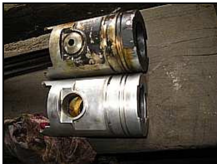
E11 – An almost completely cleaned piston contrasts with one in a just removed state. The surgically smooth finish should be worth a few extra Kilowatts at the flywheel I think.
