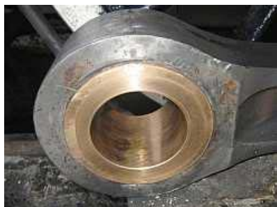
A typical bronze bushing in a locomotive application.
