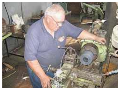
Reefsteamers Machinist James Thompson machines a new bushing for an Expansion Link Trunnion. The length of the shaving tail demonstrates how easy this material is to cut and machine on a standard lathe. No broken cutting tools here!
