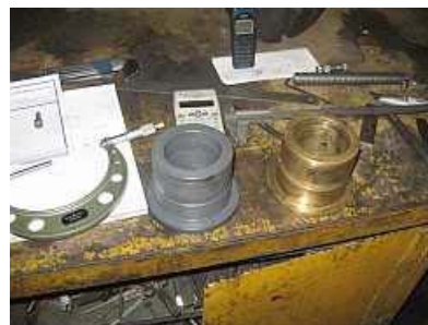
An original bronze bushing (RHS) and a newly machined Vesconite equivalent. (LHS)
