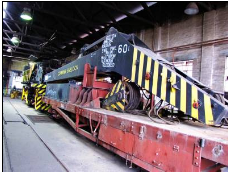
Cowans Sheldon 60ton Steam Crane. (Sandstone Heritage Trust.)
